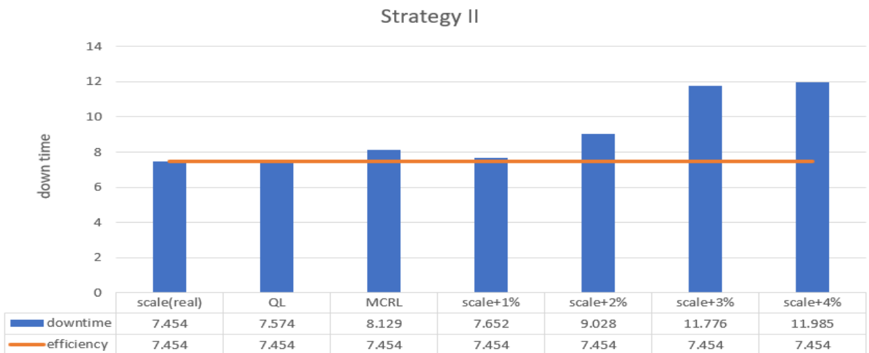
Fig. 4. System downtime of different approaches under minor changes in the Weibull shape parameters for Strategy II
